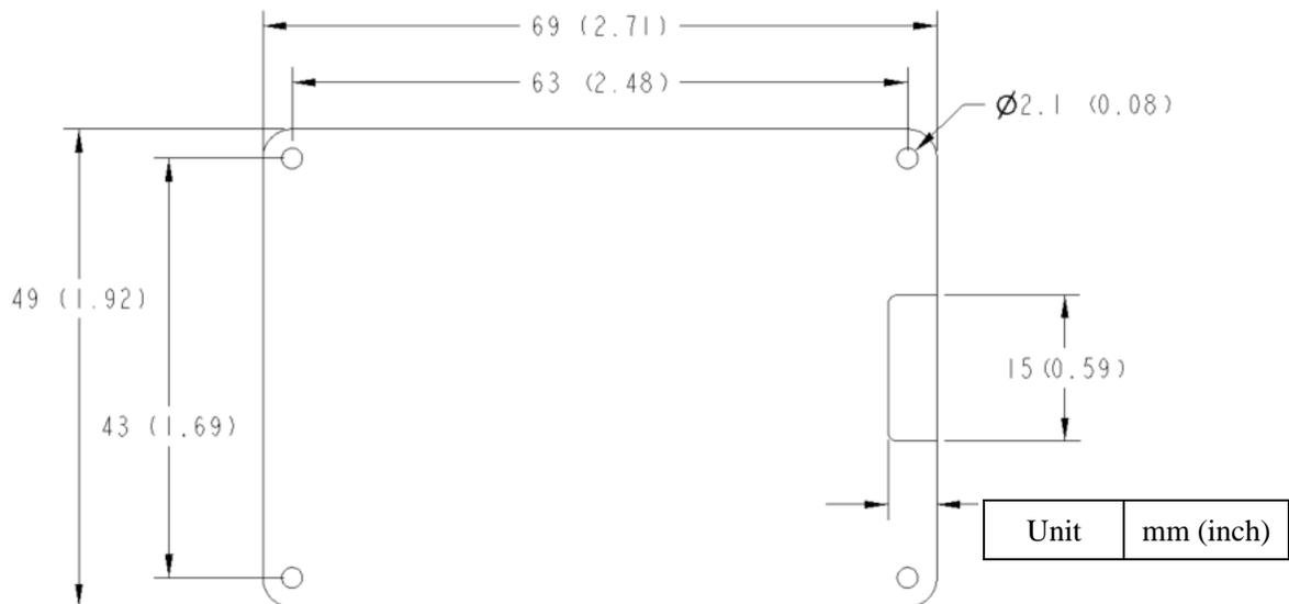
Figure 5. PCB Dimensions
