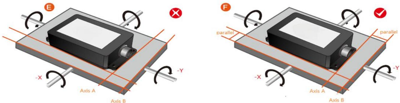
Finally, the mounting surface of the sensor and the surface to be measured must be tightly fixed, smooth in contact, and stable in rotation, and measurement errors due to acceleration and vibration must be avoided.
