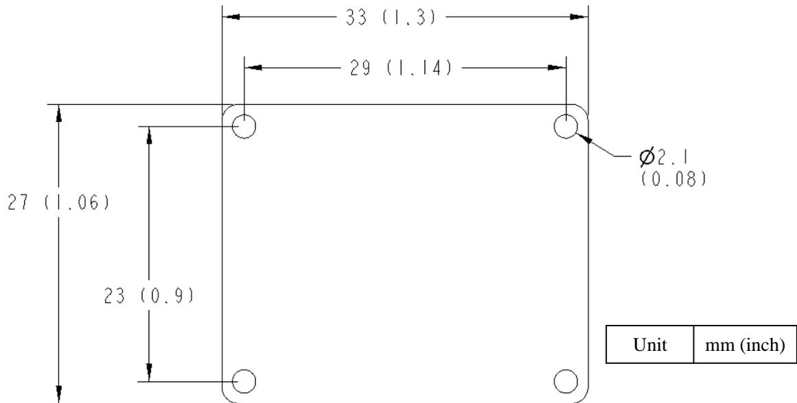
Figure 5. PCB Dimensions
